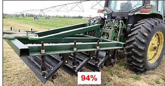
Four-stage roller/crimper. Adopted by an organic farm in Great Britain. Kornecki, 2011, US patent no.: 7,987,917 B1.
